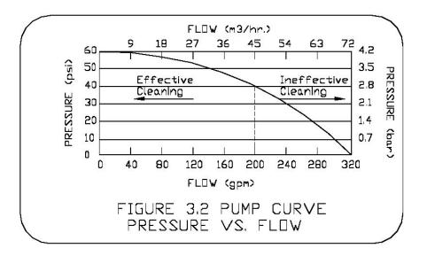
Figure 3.2 shows an example of a pump curve. Since a minimum of 40 PSI must be maintained, the critical point for this pump is at 200 gpm. Any flow greater than this will not yield effective cleaning during the backwash cycle.
