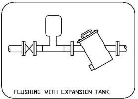
tank installed directly upstream of the filter inlet. The expansion tank would contain water at operating pressure to supply to the filter during the cleaning cycle.
